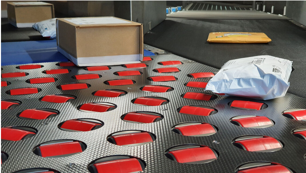
Figure 18. Example of a flow splitter for mixed mail: Siemens VarioRoute [© Siemens Logistics]
