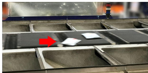
Figure 17. Typical operational issues in the automated processing of polybags: infeed problems on cross-belt sorter due to low weight [own illustration]
