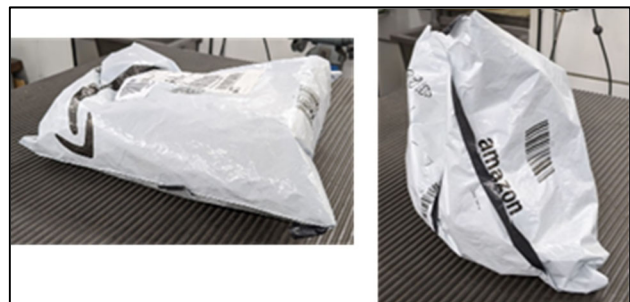
Figure 20. Change in the shape of a polybag before and after a free fall from a height of 80 cm [own illustration]
