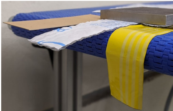
Figure 23. Flexural behavior: a) polybags without self-supporting structure, b) with self-supporting structure (air cushion), c) cardboard as reference [own illustration]
