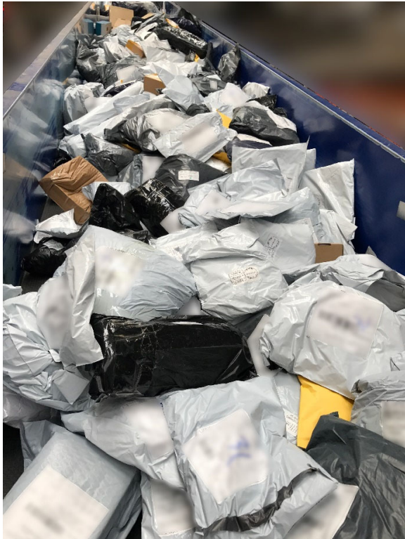
Figure 10. What looks like garbage are actually polybags after bulk unloading from the transportation containers onto a bulk conveyor and prior to singulation and sortation [own illustration]
