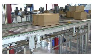
Figure 6. Synchronization conveyor (positioner), by Tansnorm System
