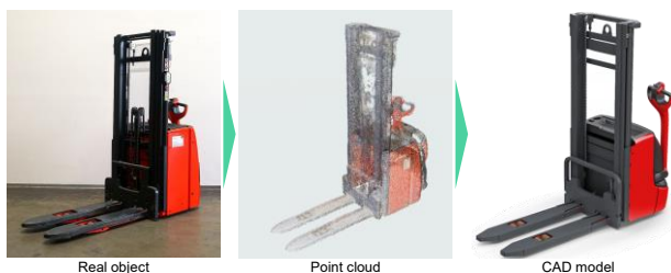
Figure 10.: From the real object via the point cloud to the CAD model
